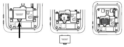
3. Replace the backup battery compartment cover. Push the large tab until it locks securely.
