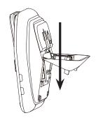
4. Rotate the wall mount bracket and lock it into wall mount position. Route the telephone line cord and power adaptor cord through the slot on the bottom of the telephone base. Bundle the telephone line cord and the power adaptor cord with twist ties.
