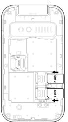
Place the SIM card with the chip facing downwards and slide it into its housing. Make sure that it is correctly inserted. To remove the card, press it and slide it out
