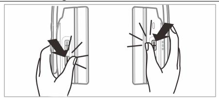
You can adjust the volume for the left and right sides of the headset independently. Press '+' button repeatedly or continuously on the desired side of the headset to increase volume and '-' button to decrease volume. The Headset will beep when volume reaches midway volume.
