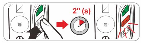
The balance can be controlled by pressing the balance button on the headphones. Press and hold this for **2** seconds, the button will light up red. At this point, pushing headset '+' button will alter the audio to the left earphone. Pushing the '–' button will alter the audio to the right earphone. At minimum, maximum or middle point a beep will be heard. If the buttons are not pressed, balance setting mode will switch off automatically after **5** seconds.
