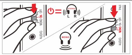
Stereo or Mono mode can be controlled by moving **OFF/ON/Mono** switch to the desired side. This switch is found on the underside of the charging base (using a needle or pencil is helpful).
