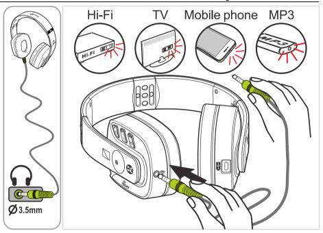
Insert one side of 3.5mm (male to male) cable jack into 'Audio' socket found on the bottom of the Headset. Insert the other side of the 3.5mm jack into audio-out socket of your Hi-fi, mobile phone, TV or MP3 player.
