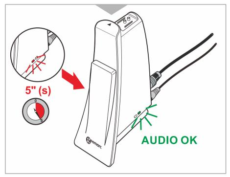
7. Place the headphones onto the Charging Base. A red light will show on the headphones. The red light indicates the headphone's batteries are charging. Charging takes 5 hours. After full charge the red light changes to green.
