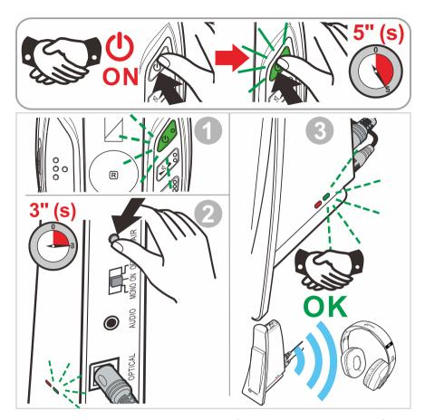
Your Headset was paired with the Charging Base at the factory so that when you switch on the Headset, it will automatically recognise the Base. However, if for any reason the Headset and Base are no longer paired, there is a very simple procedure to follow in order to pair the two devices:
