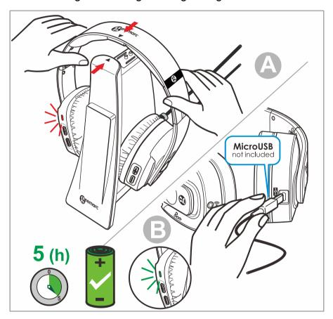
There is a Micro USB port located at the bottom of one of the earpieces. This allows charging to take place via other means. Please note the Micro USB is not included.
