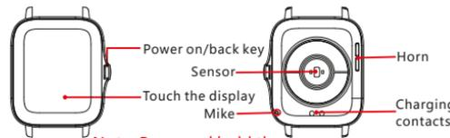
Note: Press and hold the power-on key to turn the watch on
